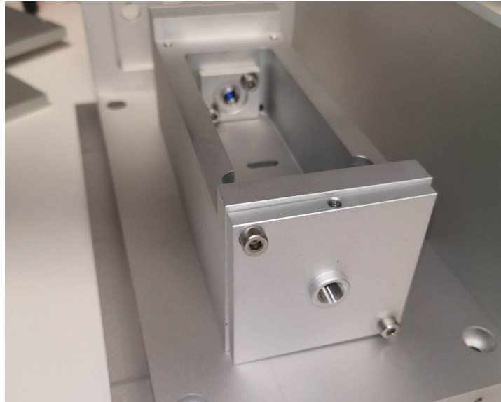
Figure 3.15: Holding plate for the recollimation lens (L3) at the front of the laser's inner housing. L3 is not placed yet. In the back, the first collimation lens L1 of the laser diode is visible.
